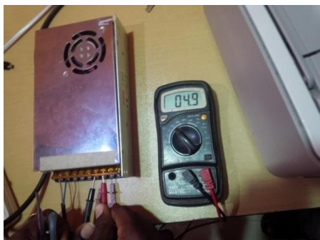
Figure 4.1 : Testing the Circuit
