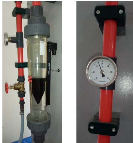
Picture 2. Thermometer and rotameter indicators
