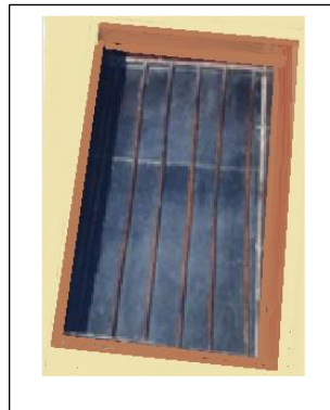
Figure 4. Photograph of the Standard Solar Heater Without Convex Lenses.
