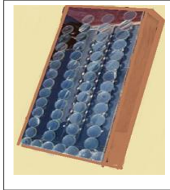
Figure 3. Photograph of the Solar Heater Equipped with Convex Lenses.
