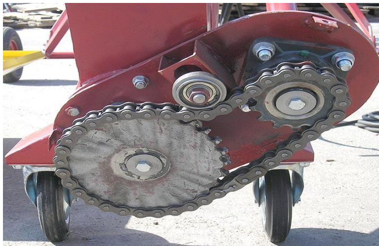
Figure 2. Distribution of the movement to several drive shafts through a chain drive.
