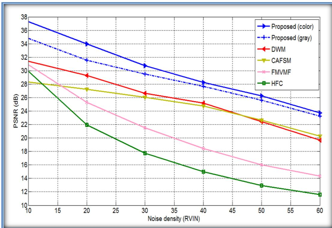
**Fig. 3: Comparison chart in term of PSNR of the proposed color image algorithm with related works using the “Peppers” image corrupted with RVIN (10% - 60%).**
