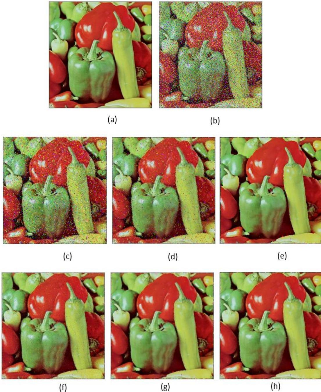
**Fig. 4: Results of RVIN removing of “Peppers” image, (a) original image, (b) Noisy image corrupted with 30 % RVIN (PSNR: 13.43), (c) Processed image with HFC (PSNR: 17.75), (d) Processed image with FMVMF (PSNR: 21.53), (e) Processed image with CAFSM (PSNR: 26.04), (f) Processed image with DWM (PSNR: 26.65) (g) Processed image with the proposed gray image algorithm (PSNR: 29.48), (h) Processed image using the proposed color image algorithm (PSNR: 30.82).**
