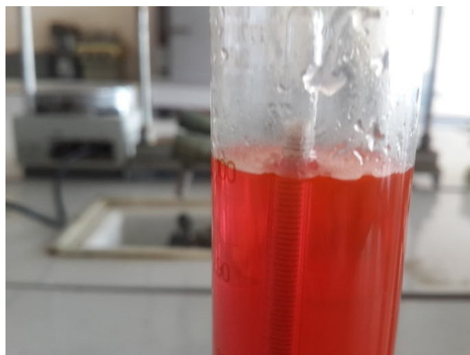
Fig. 2. Determination of the density of antifreeze
